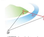
VECTOR also calculates and displays relative values between two remote objects A and B:  $\Delta r$  slope distance
