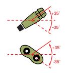
A traditional magnetic compass must be held level so that its needle can swing and point to north. The digital compass inside VECTOR gives you correct bearings even when tilted by as much as 35 degrees.
