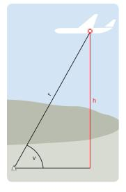
With an extended inclination range of -30° to +90° VECTOR 21 AERO allows measurements such as aircraft position and height above ground, cloud height, flight path of large migratory birds, etc.
