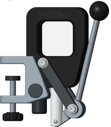
The 24 mm piston is chromed and rectified and runs inside a bronze bushing adjusted to achieve maximum smoothness and very reduced tolerances. The machined parts of the piston are subsequently blued to avoid any rust phenomena. The light alloy parts are anodized. The lever is made of stainless steel, as well as the pin nuts. The knob is made with a real billiard ball of the famous Belgian brand Aramith.
