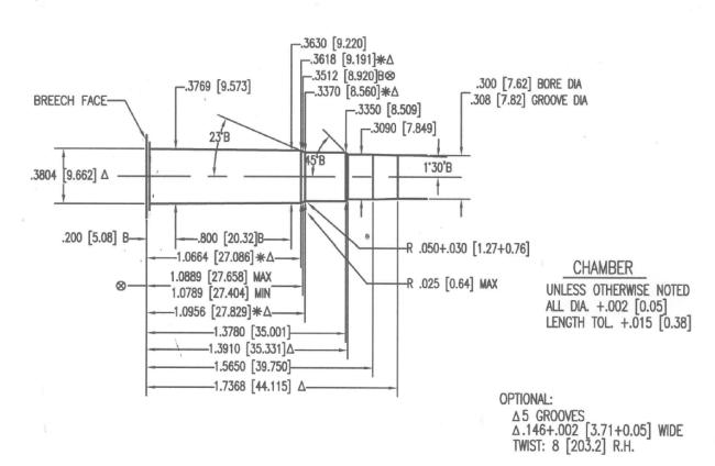
MIN. BORE & GROOVE AREA: .0737 SQ. IN. [47.548 mm²]
